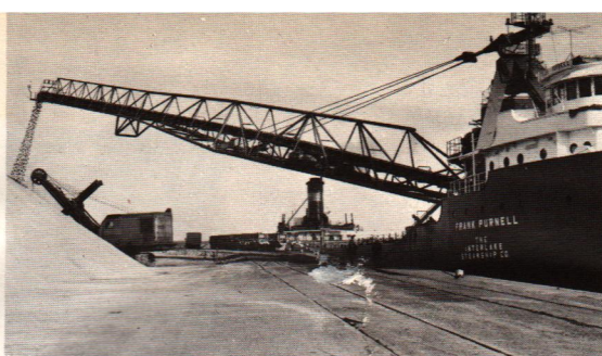
The 250-foot conveyor boom of the Interlake Steamer Frank Purnell can swing to either side of the ship and discharge up to 14,200 tons of cargo at 5,000 tons per hour.
