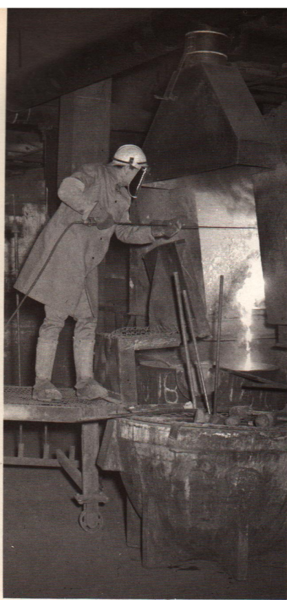
Massive Manganese is tapped from one of 15 cells that electrolytically produce the high-purity metal in massive form at PM's Manganese Chemicals Division plant, Kingwood, West Virginia.
