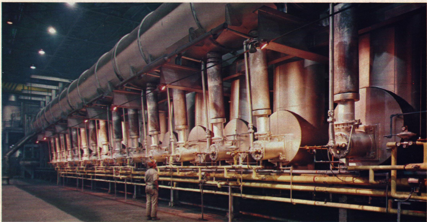
Cake tumbles into "green balls" in a balling drum. One of the three 310' long indurating lines which bake the green balls in 2,500°F temperature converting them into dry, hard pellets.
