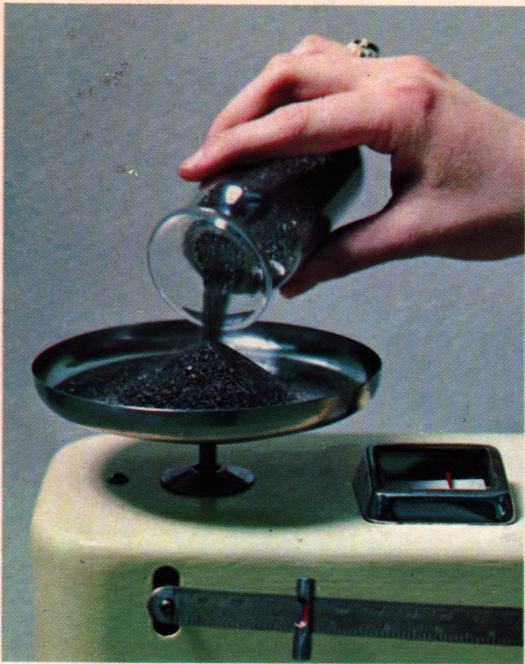
Iron ore concentrate from Wabush, known as Specular Hematite is heavy, black and sparkles much like graphite.
