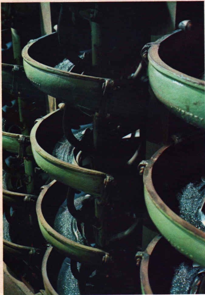
Spiral Separators (note sparkling concentrate).
