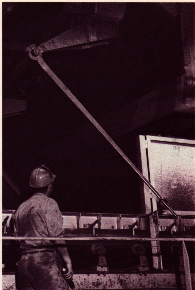
Cake tumbles into "green balls" in a balling drum. One of the three 310' long indurating lines which bake the green balls in 2,500°F temperature converting them into dry, hard pellets.
