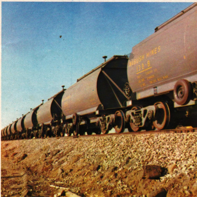
The auto wheel clearly shown on the side engages a raised rail to open the bottom doors. An identical wheel on the other side will close the door.
