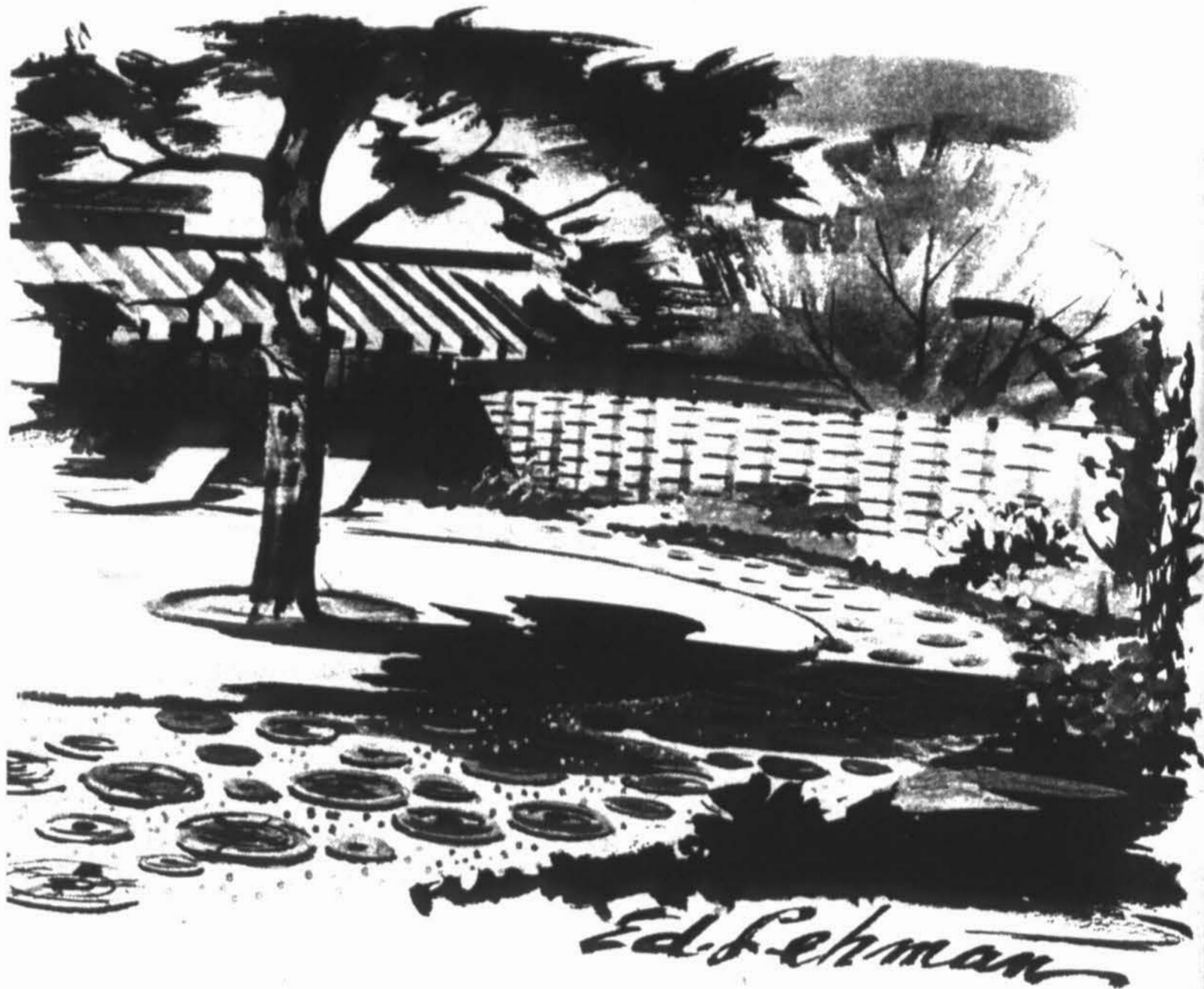
FORTHAT BACK GARDEN - Crosscut logs make fine paving blocks if you like an informal look on your terrace. They're nice to step on in bare feet or heels. And they can be set in concrete, sand or sod without much trouble. Have the lumberyard cut logs in sections three or four inches deep. Dig a trench almost the depth of the sections and set them on end as close together as you wish. Then fill in the trench with concrete, sand or topsoil. Allow wood tops to protrude a little but not enough to trip over. Wash them off with a hose. If you want sod between the logs sow seed so grass will be level with wood and the lawn mower can pass smoothly over the tops of both. For greater durability treat logs after they have been cut with wood preservative - (Barbara Barnes).
